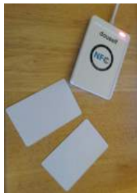
(b) ACR122U reader with two of three Mifare DESFire EV1 cards
